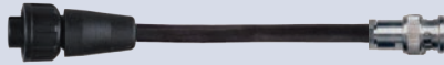
052 Cabling - Polyurethane Jacketed Polyurethane cable, 2-conductor twisted pair w/ drain, shielded (-50 to +121 °F). Shown with BNC connector to 2-pin MIL
