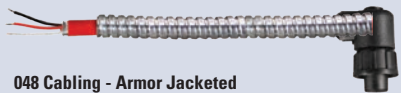
048 Cabling - Armor Jacketed High temp FEP Cable, Armor Jacketed, 2-conductor twisted pair w/ drain, shielded (90 to +392 °F). Shown with Right Angle 2-Pin MIL connector
